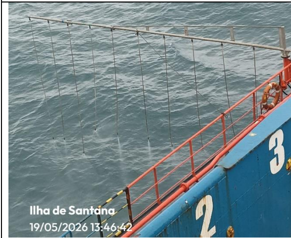
Teste Fire Fighting System (FiFi) bombordo
