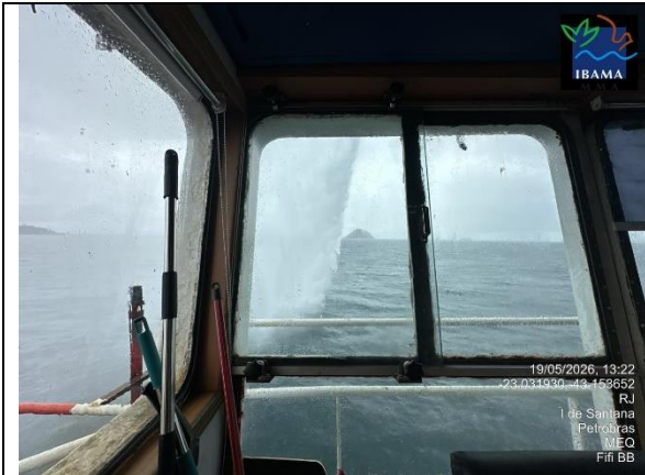
Teste Fire Fighting System (FiFi) bombordo
