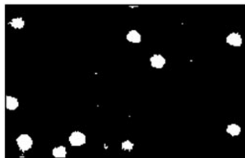
Figure 2. The tracks of alpha particles formed on LR-115 plastic track detector
