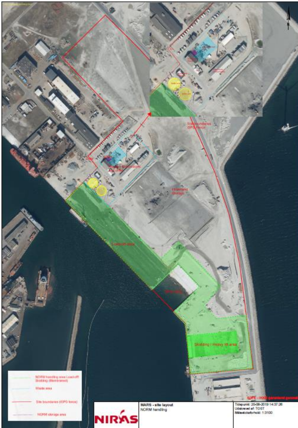
The purple square is dedicated for NORM storage, Green areas annotate NORM handling area
